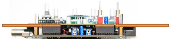
Note the gaps between the female connectors and the upper pc board
