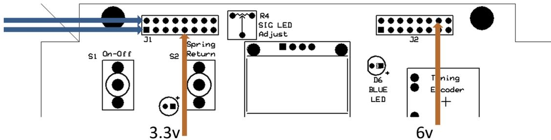
**Note: The blue arrows points to the 12V pins and the orange arrows point to the 3.3V and 6V pins.**
