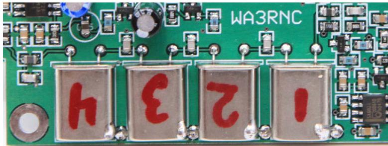
Mount the crystals down tight against the board. Solder and trim 8 leads. Ground the crystal cans with wires cut from the included sacrificial resistors. Do not overheat the crystal cans! Be quick when soldering to the cans. Trim the grounding wires. The resistors may be discarded.
