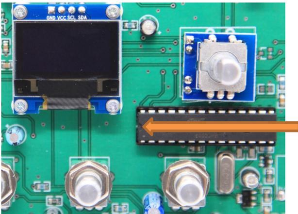
***Note the orientation notch above that the arrow indicates.***
