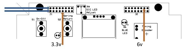
Note: The blue arrows points to the 12V pins and the orange arrows point to the 3.3V and 6V pins.
