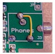
allow both headphone earpieces to play, but only if you never intend to use a mono plug connected to the "Phones" jack. To make this mod, the top case half must be removed by removing all the knobs and the four nuts holding the case half to the board assembly. Remove the four black case screws and lift off the upper-case half. Carefully solder in a jumper wire as shown in yellow in
