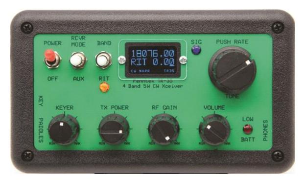
The TR-35 is a 4-band 5-watt CW transceiver covering the 40-, 30-, 20-, and 17-meter bands with generous receiver tuning ranges above and below each band. Selectable receiver modes allow for narrow band CW, wideband CW, and SSB reception.
