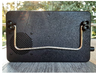
Tilt bail shown collapsed.
