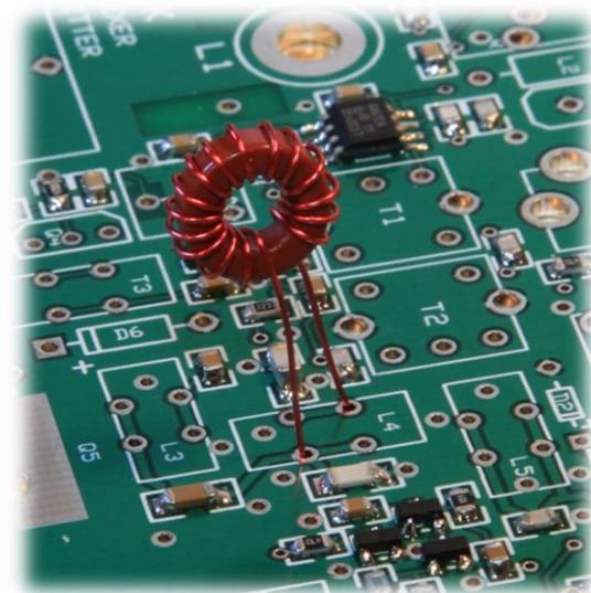
**Note: The previous photos show the toroids standing above the board. This is to show the two different mounting options. All of the coils are mounted down against the PC board.**
