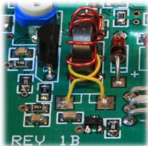
a piece of the magnet wire for this winding. (The photo shows the secondary winding with yellow wire for clarity.)
