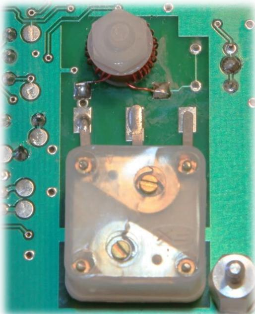
L1 leads are soldered to the pads as shown in the photo to the left.
